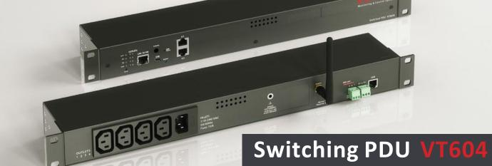
Device is used for load management and allows to switch on/off or reboot up to 4 outlets. It has built-in temperature sensor, two ports for analog sensors, two dry contacts, two12V outputs for devices, USB port for camera, a slot for GSM modem and allows to connect up to 4 IP cameras.
