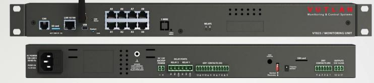
The unit is used in data centers, remote & industrial facilities, offices. Can connect up to 30 sensors, 12 dry contacts, two 12V alarm beacons, GSM modem, USB-cam, SD card, 1-Wire board (instead of VT18) for reader connection.
